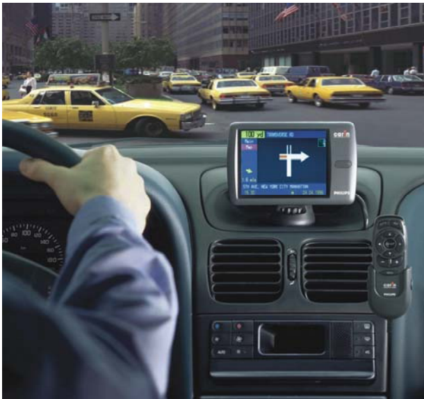
The Carin 550 navigator has a 5" screen, GPS, and motion-sensing technology.
